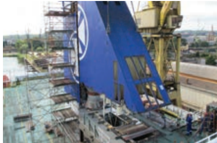
A Scrubber installed onboard a DFDS Seaways vessel.
